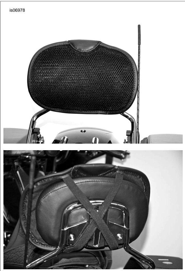
Figure 2. Circulator Wide Sissy Bar Pad Installed
